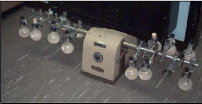
Figure 2. Batch experiment set up showing wrist shaker.
